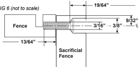
**Note:** The counter bores allow the fixing screw heads to sit well below the sacrificial fence surface when fitted to the fence.
