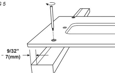
Through drill the 2x fixing holes using a 3/16" (5mm) drill bit.
