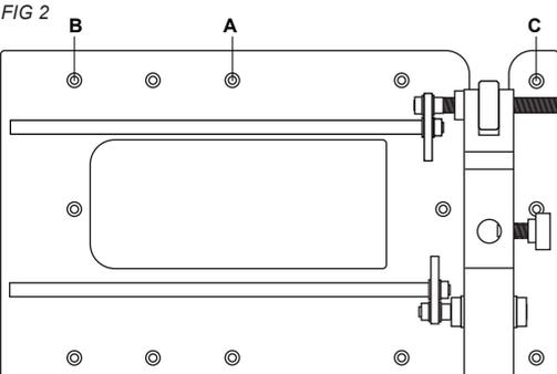
The Side Fence fixing position is determined by the desired distance of the routing pass from the edge of the workpiece (See Fig 3)
