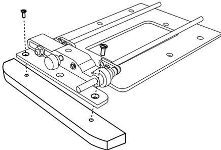
Slide the router back onto the CRB7 rods and position it in the approximate area of the desired router pass.
